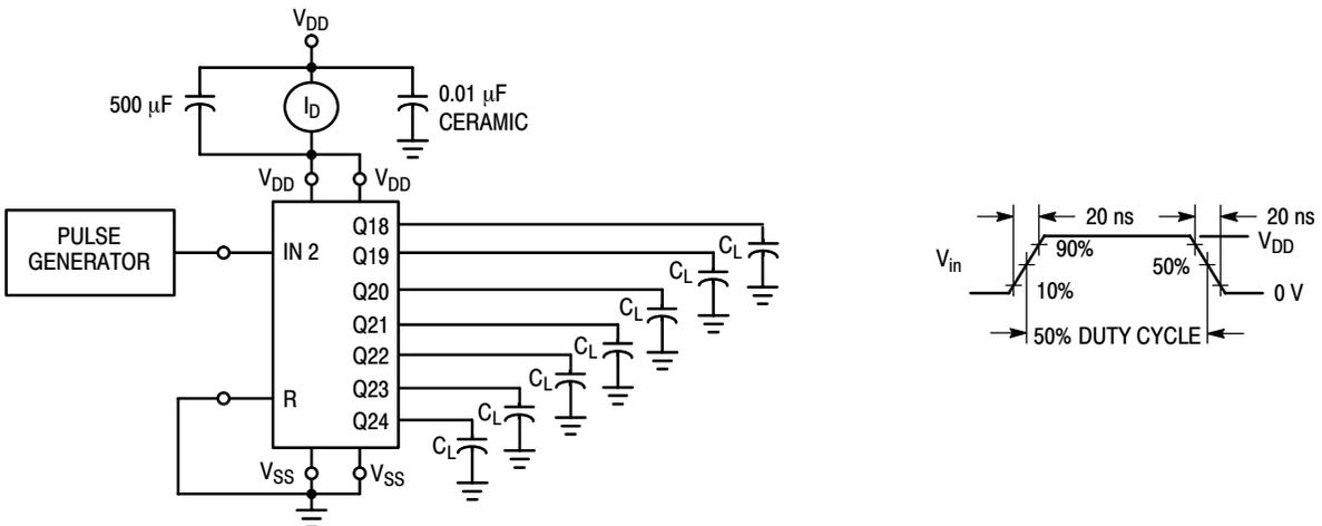
Figure 1. Power Dissipation Test Circuit and Waveform
