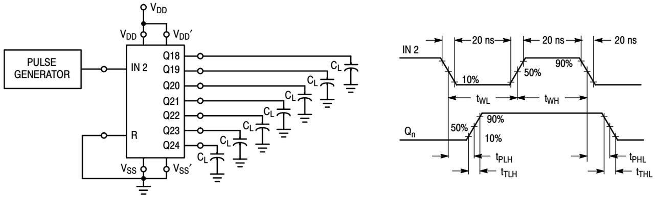
Figure 2. Switching Time Test Circuit and Waveforms
